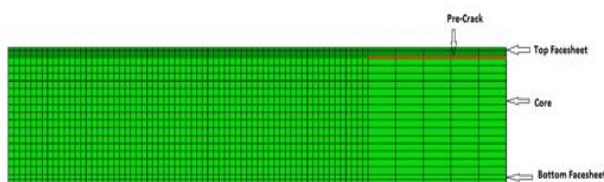
Figure.2. DCB Mesh Discretization
